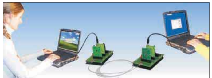
One way data transfer between two computers through optical fibres
