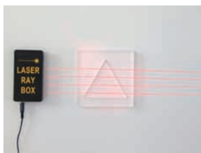
ray tracing through interface glass-to-glass
