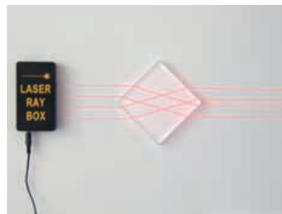
turning of light beam by cube
