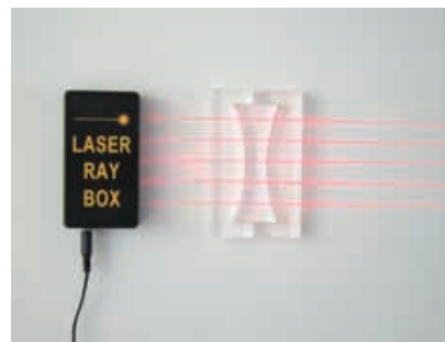
concave lens with interface glass-to-glass
