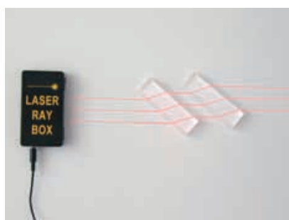
ray shift by planparallel plates
